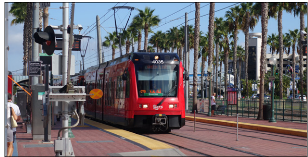
Figure ES-6: LRT Low-Floor Example: San Diego Trolley
