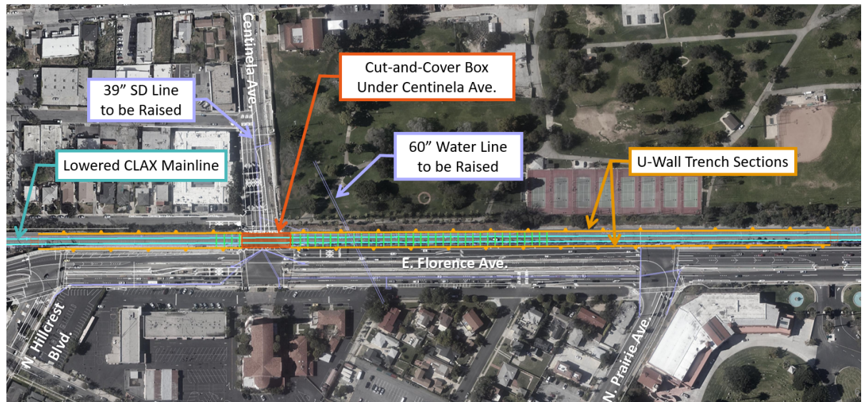
Figure 2-7. Alternative 2 – LRT Below Grade
