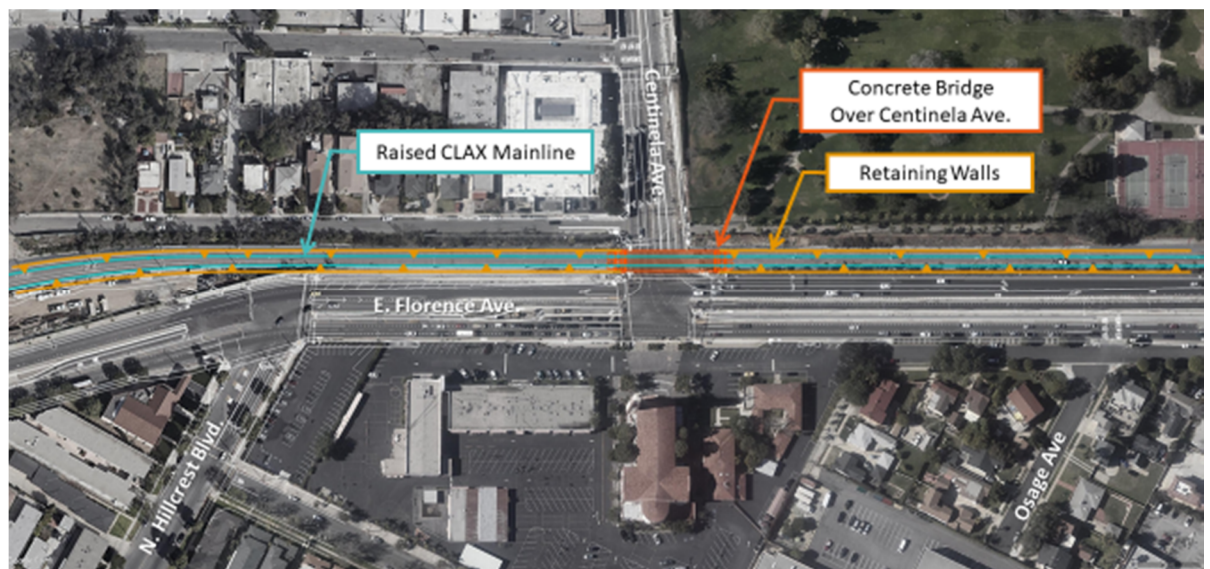
Figure 2-6. Alternative 1C – LRT Above Grade without Shoofly
