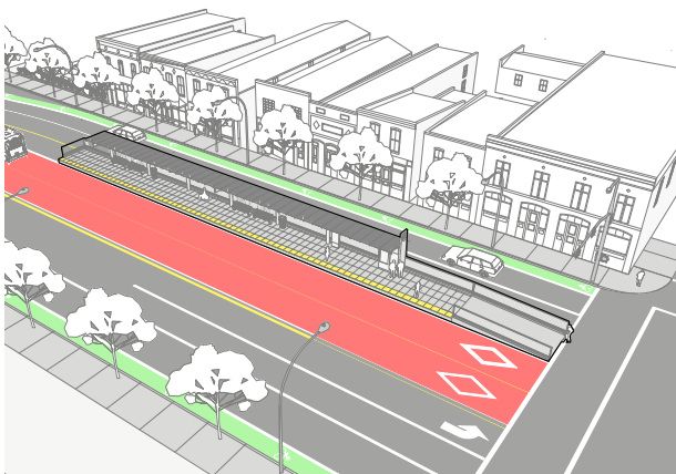
Center Running – Side/Side Staggered Station
