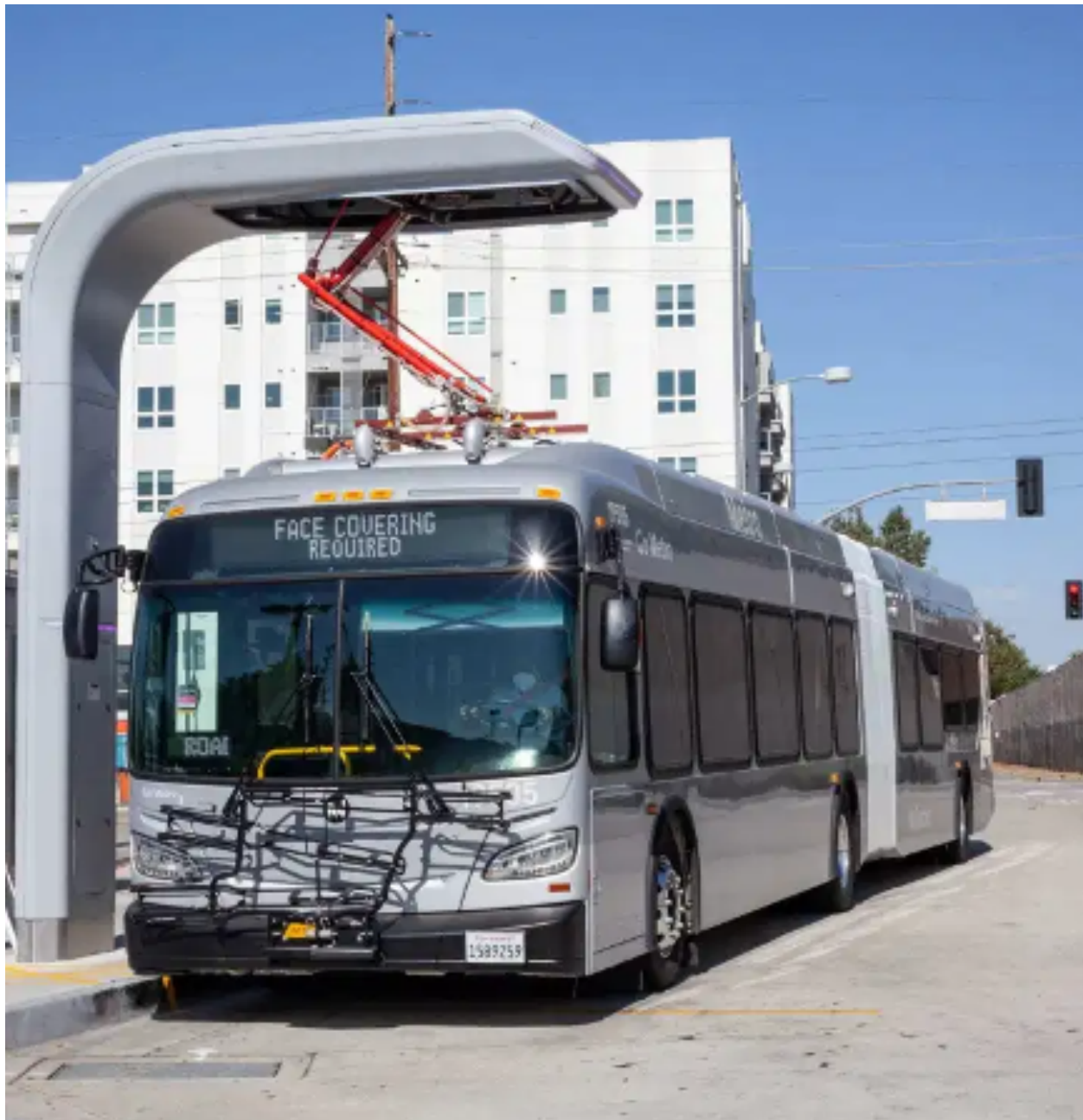
Figure 3-4. North Hollywood Station On-Route Charger
