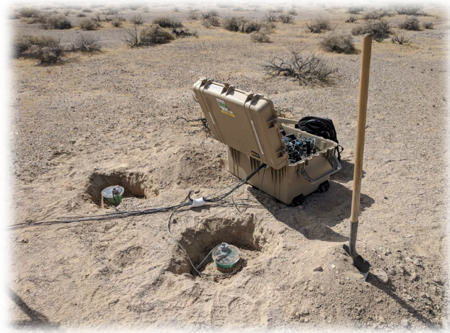
Caption: Two portable sensors: a strong motion sensor (to record strong shaking that can be felt) and a broadband sensor (to record weak motion for detecting small earthquakes) buried into the ground to detect earthquakes. These stations can be quickly deployed and send real-time data back to the USGS via cellular telemetry immediately after they are installed.
