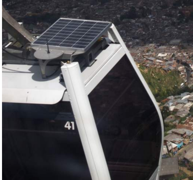
Image 37 – Solar Panels Mounted to Cabin Roof
