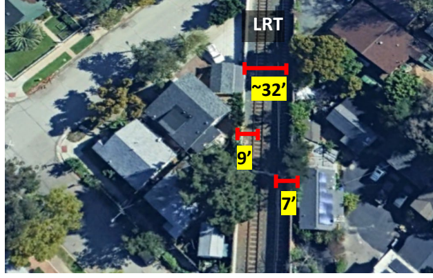
A Line, South Pasadena (LRT) ~7' to 9' property line to LRT centerline ~30' LRT corridor
