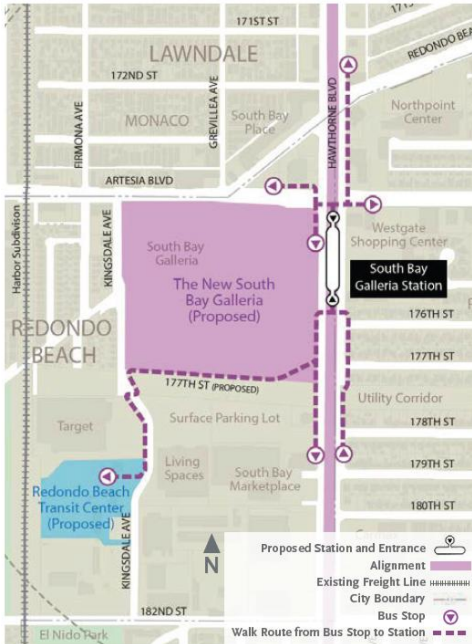
Diagram of pedestrian connection between proposed South Bay Galleria station and Redondo Beach Transit Center (Urban Design Report, 2023)
