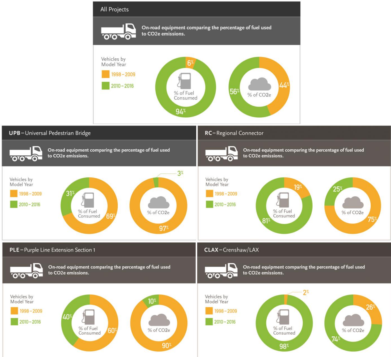
Figure 6 –Projects summary for emissions reductions (CO2e) based on Tier 4 equipment rather than Tier 2 equipment.
