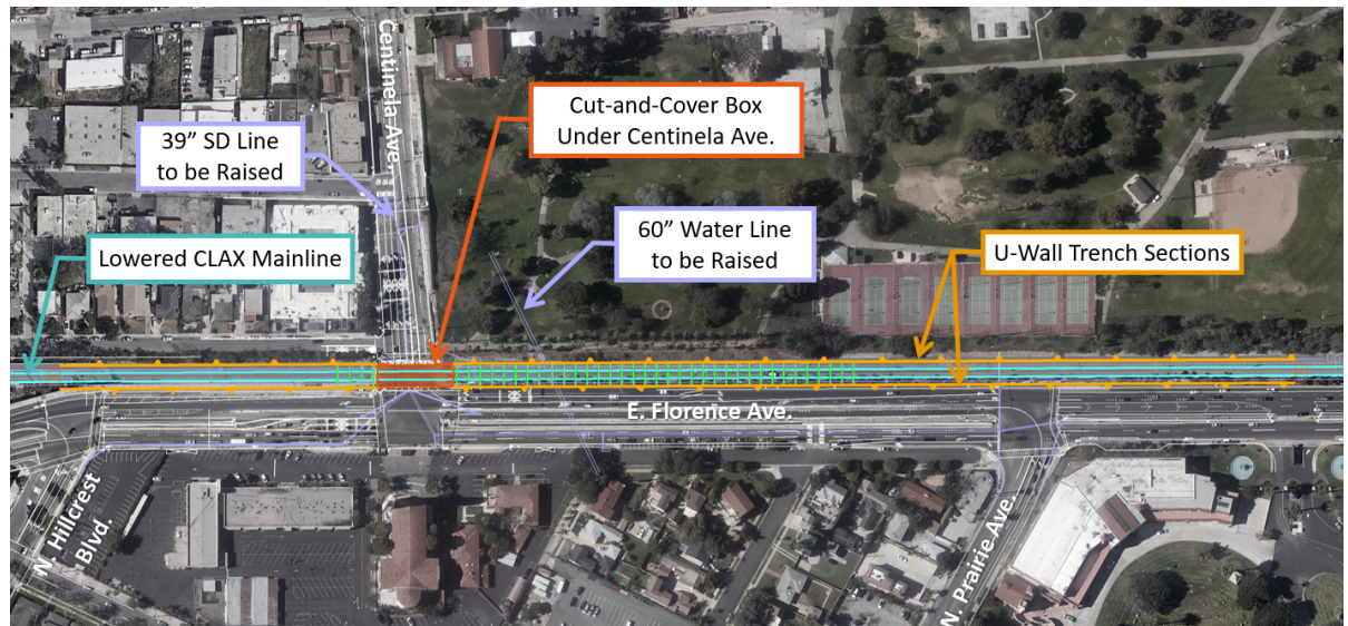
Figure 2-7. Alternative 2 – LRT Below Grade
