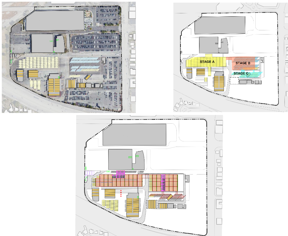
Figure 3-17. Division 9 – Existing, Construction Staging, and Buildout
