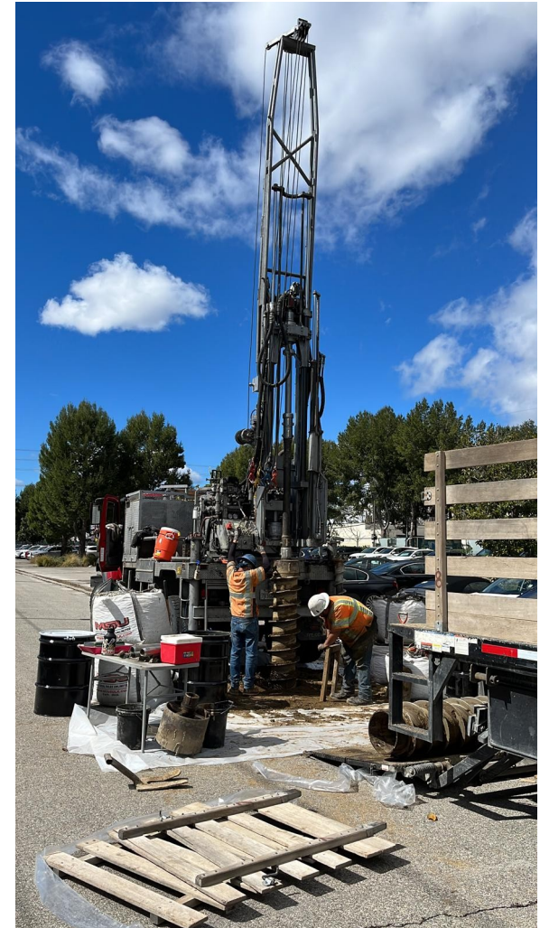
Geotech- percolation testing for stormwater capture scope
