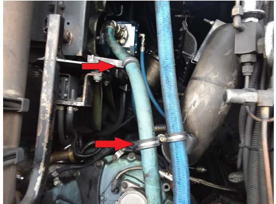
Hydraulic fan oil line securement
