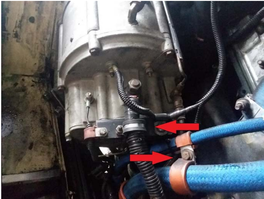
Alternator cable and hydraulic oil line securement
