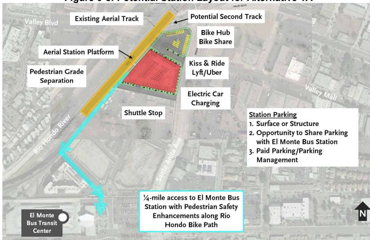
Figure 0-8: Potential Station Layout for Alternative 1A
