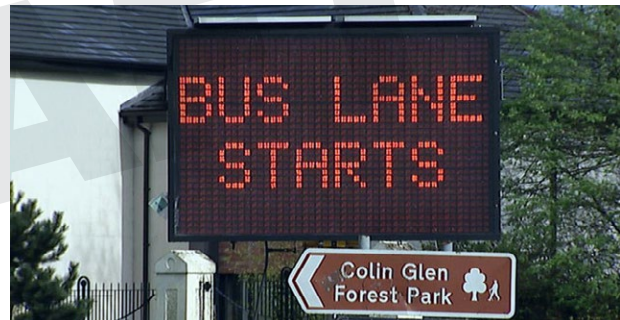
Electronic signage can dynamically manage BRT Guideways in a variety of conditions / Source: ITVhub
