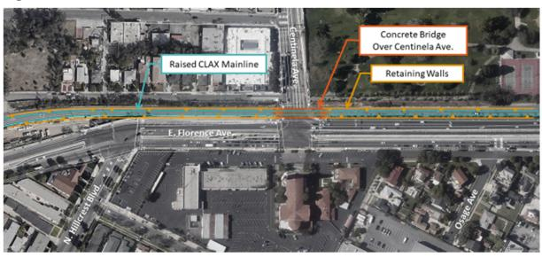
Figure 2-1. Alternative 1A – LRT Above Grade
