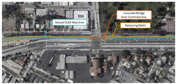
Figure 2-6. Alternative 1C – LRT Above Grade without Shoofly
