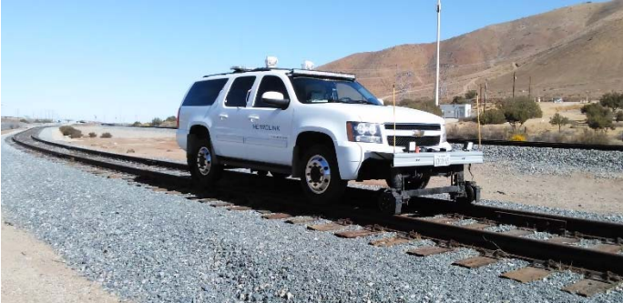
Picture 1: One of two SCRRA Hy-Rail Vehicles used to complete the field visit with MTA.
