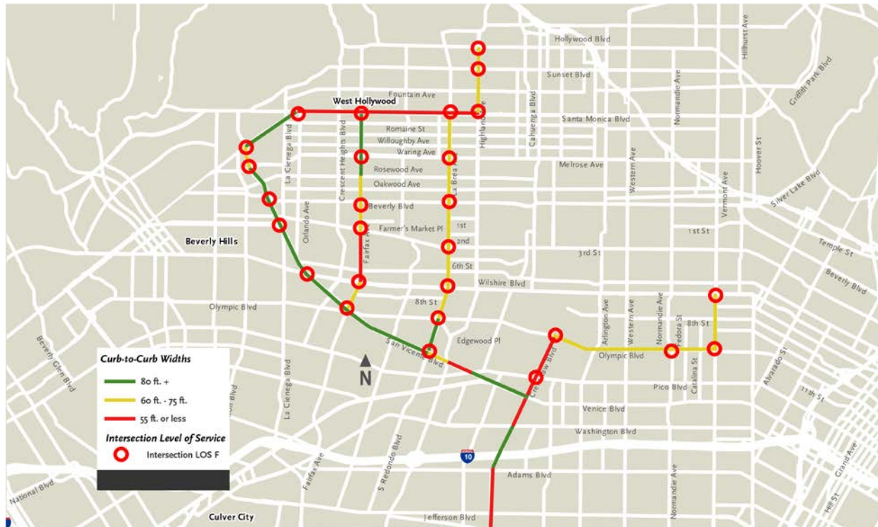
Figure ES - 18 – Alignment Constraints: Right-of-Way and Required Grade Separations at Congested Intersections
