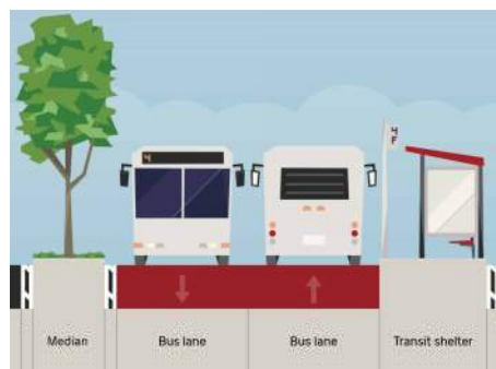
Median layout at BRT station
