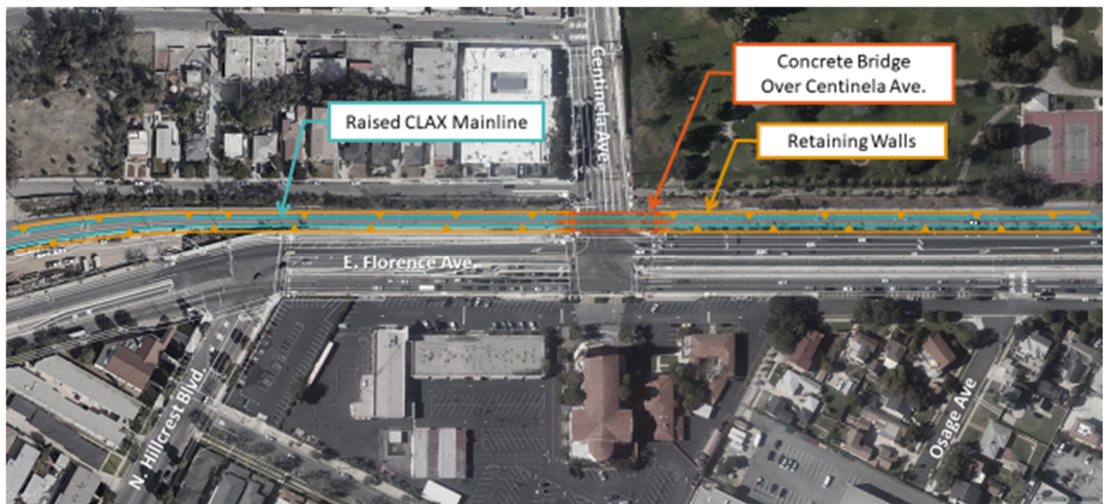
Figure 2-1. Alternative 1A – LRT Above Grade
