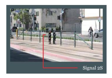
The normal and reverse running signals 2S & 4S are installed side-by-side, and are located in the approach to the 21st Street intersection. A traffic Bar Signal is located at the far right corner of the intersection, and operates independently of the interlocking signals. The ROC Controller SOPs indicate that this interlocking does not have an "Automatic" mode and that during normal operation, the interlocking remains in "Central" mode with signals 2S and 4N fleeted.
