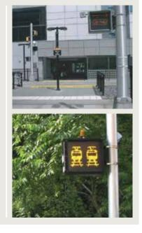
The use of "Second Train Signals" is effective in advising motorists and pedestrians that two trains are approaching an intersection. This is an active sign that illuminates when one or two trains are approaching. The sign may be a blank-out LED sign or it may use flashing lights or another type of indication (such as backlit illumination) to an otherwise static sign. TWG is advised that Metro has installed these signs at a number of locations.
