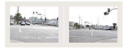
There are no street markings or channelization to guide pedestrians to cross the tracks, and pedestrian street markings are fading and need to be repainted.
