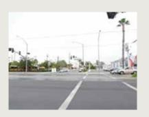
There are no street markings or channelization to guide pedestrians through the crossing. Further, there is no street marking or treatment to mark the edge of the crossing.
