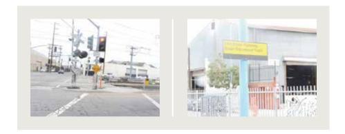
This intersection includes most of the basic vehicle and pedestrian signs, with the exception of the "No Vehicle on Track" sign and "Do not Stop on Track" sign.
