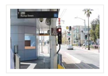
The Stop Signal Working Group made a number of observations related to the angle/orientation at the various signals. Further, the group questioned if the 500 feet sighting distance requirement is satisfied at signals 2S & 4S.
